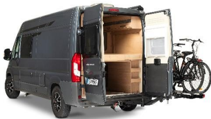
Caption 2: Access to the rear doors is always possible, even with the rear carrier system, thanks to the swivel function.
