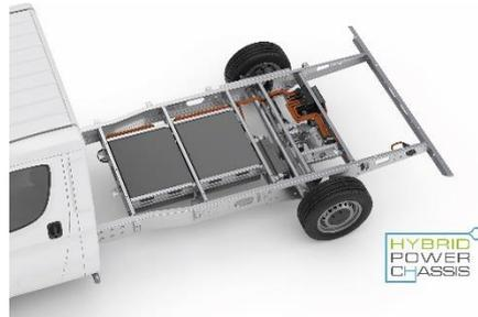
The Green Trailer platform undergoing testing. The aim: A 48 V solution with the added benefit of range optimisation, improved carbon footprint and intelligent comfort functions at reasonable prices.
