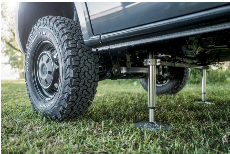
Caption: Whether on inclined angles, gravel or uneven ground, the LevelM Pro 4x4 levelling support system ensures stability and safety at all times. © AL-KO VT
