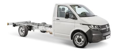
**Caption 3:** With the AL-KO lightweight chassis, the Volkswagen Transporter reaches 3.5 t gross vehicle weight. This theoretically provides 300 kg more payload. © AL-KO Vehicle Technology Group.
