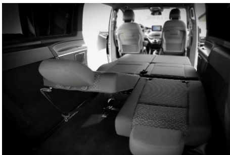
Caption 2: Each backrest allows continuously variable adjustment.
