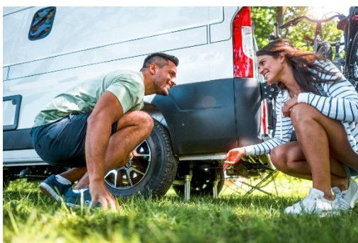
Captions: LevelVan – the first hydraulic levelling support system with carbon cylinders for vans with a net weight of less than 50 kg. © AL-KO Vehicle Technology Group
