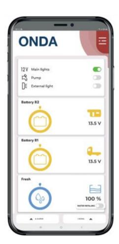
**Caption 3:** The ONDA gateway connects many functions and devices on board, including the display of the inside and outside temperature, the water level in the tanks and the battery charge level.
